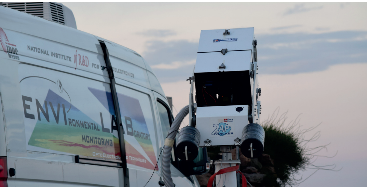
Mobile laboratory for atmospheric measurements during Pre-Tect campaign in Crete, Apr. 2017 – daytime observations of marine aerosols and clouds with the scanning UV polarization lidar
