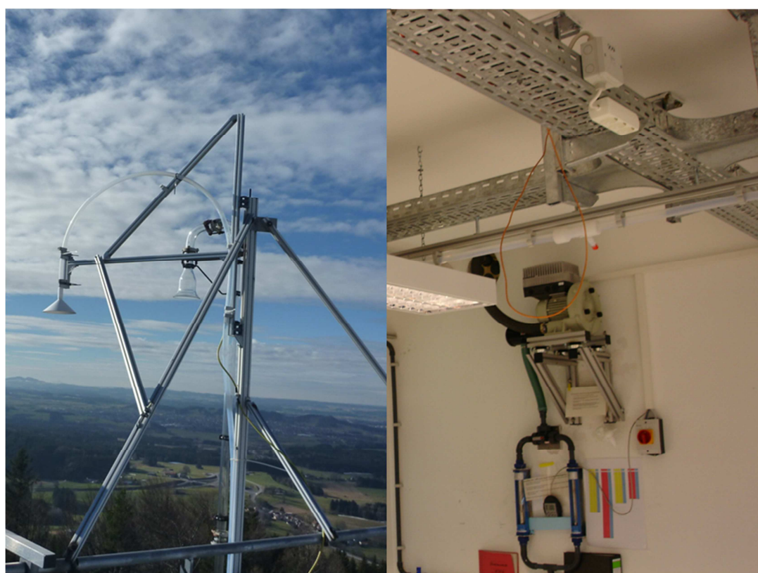
Figure 2 left: Air inlet of the guest manifold on top of the MOHp measurement platform. Right: pump set-up at the end of the manifold to enable ambient air flows up to 200 l/min.
